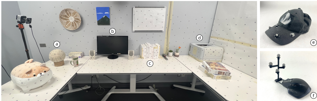
Figure 10: Setup of the experiment environment and apparatus: (a) monitor representing a user-facing flat surface; (b) printer and the surrounding wall representing far oblique surfaces; (c) bookshelf representing irregular surfaces; (d) lamp-shaped sculpture representing curved surfaces; (e) hat (for head tracking needed for Perspective Cursor); (f) mouse.
