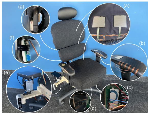
Figure 2: Chair sensors and projector actuation: (a) FSRs on back and seat for posture sensing; (b) copper tape on armrest edges for touch input; (c) circuit board and Arduino under seat; (d) Raspberry Pi under seat; (e) custom mount under right armrest to support depth camera and steerable pico projector; (f) IMU on back tracks tilt; (g) battery bank.
